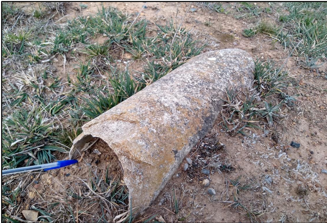
Photo 11: Potential asbestos containing material pipe
